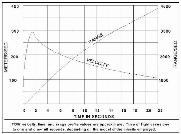
Figure 5-14. TOW Missile Flight Profile
