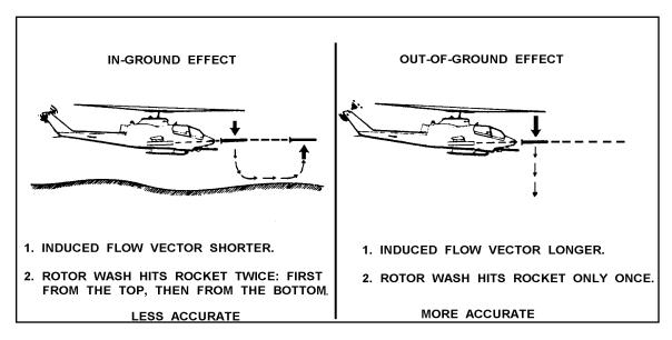
Figure 4-2. Rotor downwash error
