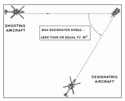
Figure 5-12. Maximum Designator Offset Angle
