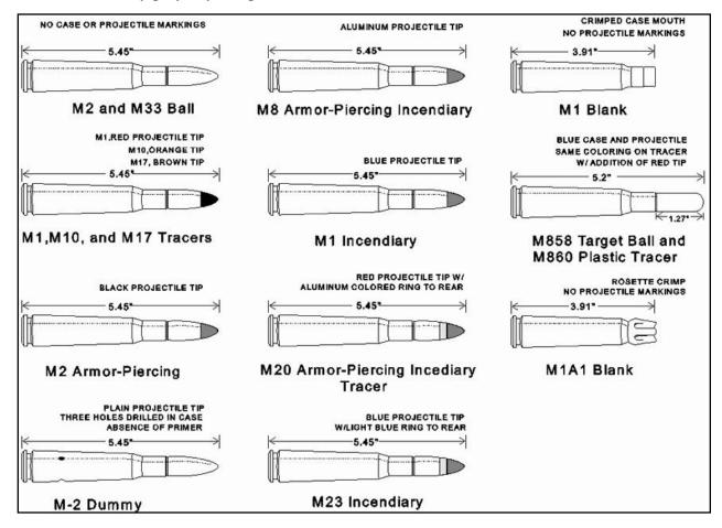
Figure 5-2. .50-caliber munitions
