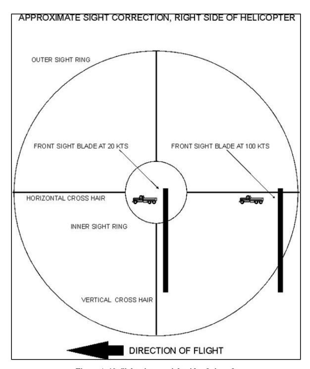
Figure A-10. Sight picture, right side of aircraft
