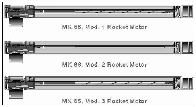
Figure 5-5. MK 66 rocket motors
