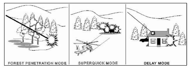
Figure 4-4. M433 multioption fuze/2.75-inch high-explosive warhead
