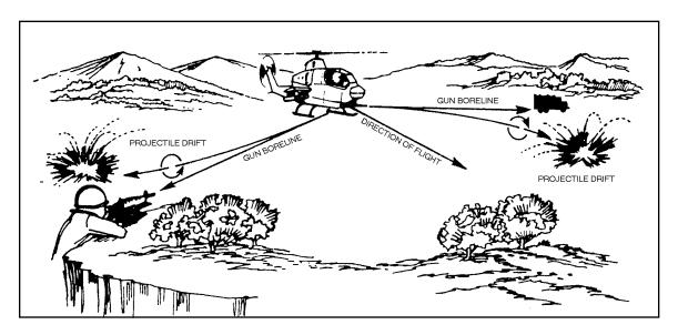
Figure 4-1. Projectile drift
